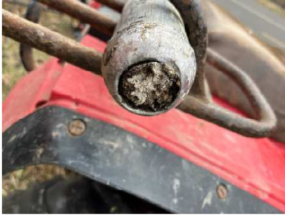
Rock in sampler cutting shoe, refusal at LGP-4
